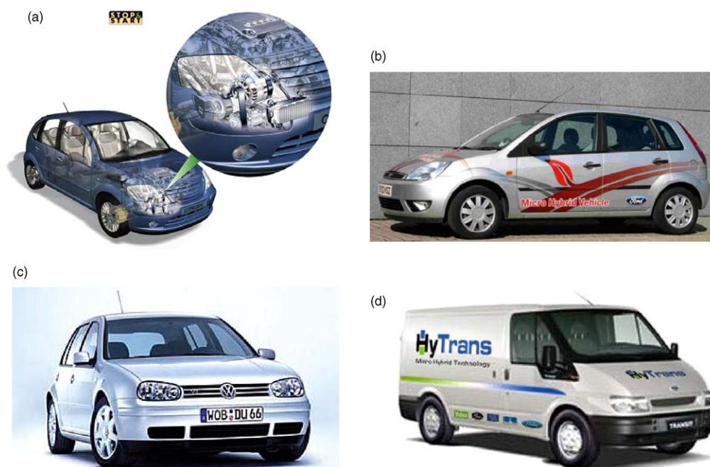
Fig. 11. Micro- and mild hybrid vehicles for the demonstration programme: (a) Citroën C3 Stop & Start, (b) Ford Fiesta Microhybrid, (c) Mild hybrid VW Golf and (d) Mild hybrid Ford Transit van.
